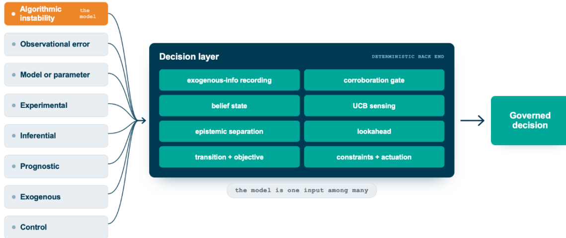
Figure 2. Eight sources of uncertainty converge into the deterministic decision layer, and the language model is one input among them, never the place the others are resolved.
